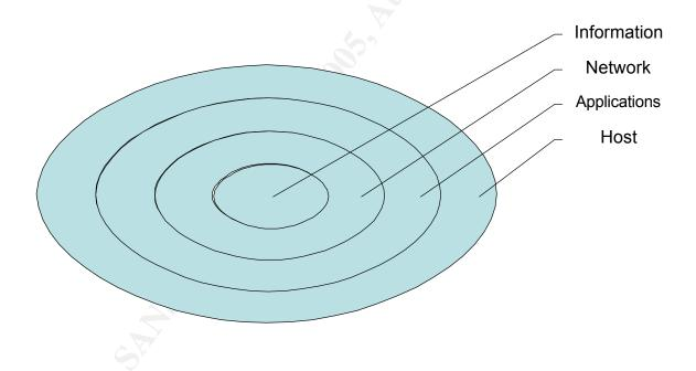
As described in [2], the diagram above represents the layers of defense for computer network. To get to the information on your computer an attacker has to penetrate the network layer (router firewall, router password, wireless security e.g. WEP, WPA), host layer (user password, user privileges, OS security), application layer (personal firewall, anti-virus software, anti-spyware software), information layer (password protection, file and directory access rights e.g. write-protection).
