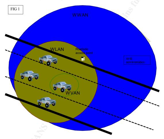
Basically an Automated Highway System is made up of three security zones represented as concentric rings in Fig 1, the Wireless Vehicle area network(WVAN), the wireless local area network(WLAN) and the wireless wide area network(WWAN).
