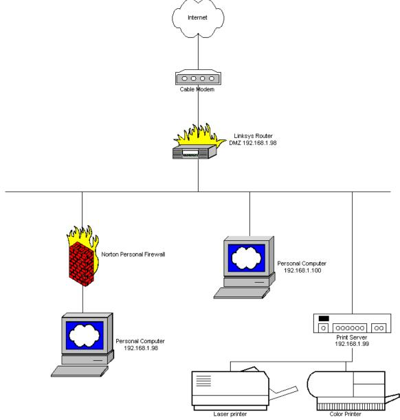
needed to be sure to set the printer server to a non-dynamic address so that the computer would always find it at 192.168.1.99. Also, my computer needed to be at a fixed address to be able to use the DMZ feature of the Linksys router, so it got assigned an address of 192.168.1.98. However, the rest of the network I wanted to be dynamically assigned, so I ran the DHCP server and set it to start at 192.168.1.100.
