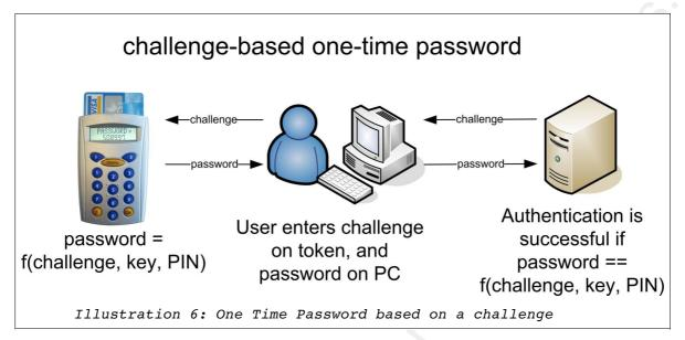
The system is based on the fact that with the possession of the challenge and the password, it is unfeasible to recover the key or the PIN, or to produce valid responses (passwords) for other challenges.
