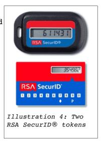
RSA SecurID<sup>3</sup>, are another type of one-time passwords. In such a system, the password changes every minute or so, by an algorithm known to the system and the user's authentication device (something you have).
