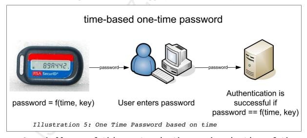
One challenge of this system is the synchronization of the time (CryptoCard Corp., 2006). The authenticating server has to cope with the drift of the internal clock of the device by computing several passwords with different times (+/- a couple of seconds). Therefore, multiple password will be accepted as correct. Another problem might be the pre-initialized key by the
