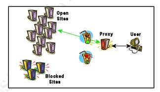
How a proxy works: When a client system requests access to a resource, it makes the request to the Proxy rather than directly. The proxy can then determine if it is acceptable based upon rule-sets. If it is, the proxy handles all transactions. The client never directly contacts the destination.
