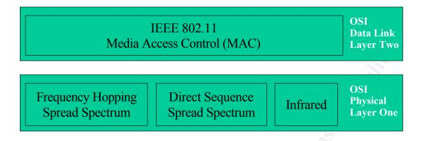
Figure 1: The OSI model according to IEEE 802.11 protocol.
