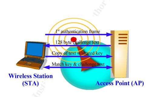
Figure 2: Graphical illustration of the shared key authentication process.
