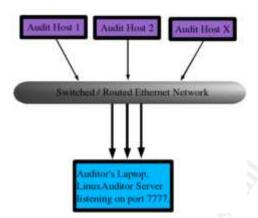
This graphic exemplifies how three audit hosts can write back to a single auditing machine and a single database. If desired, multiple audit hosts are able to write back to a single auditing machine running multiple database instances of the audit database. This type of configuration may be useful when the auditor desires to isolate subnets to a different audit database. The graphical configuration of such a setup is shown below.
