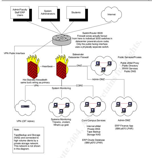
The next figure more accurately shows the physical architecture. The diagram is greatly simplified. The components included are to help illustrate the role the switches play and the issues regarding security.
