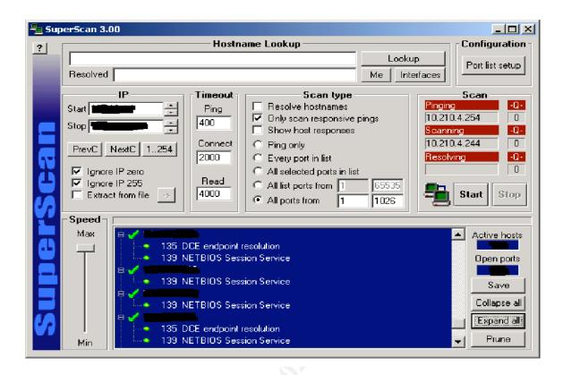
Neither scan detected any systems that appear to be a router or a network switch. The scan detected a number of PC's running Microsoft windows, printers, LAN servers, the corporate billing system and the internal mail server. From these results we have reasonably verified that no additional network connections into the ABC Company are present.
