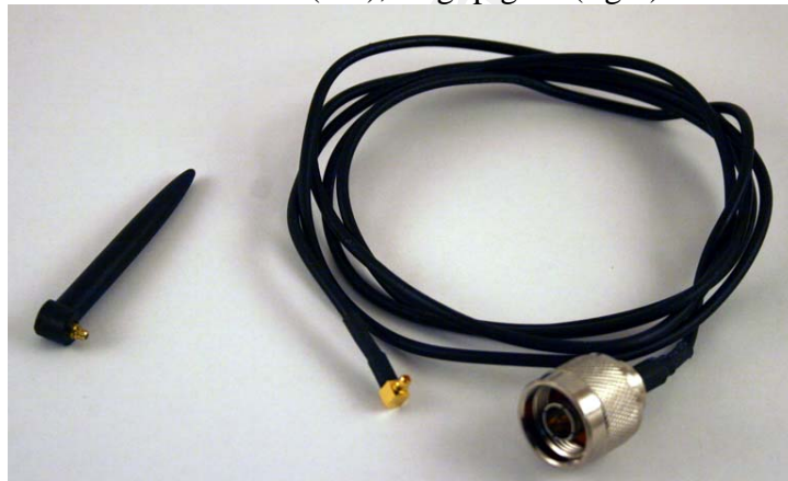
Figure 17 – Omnidirectional Antenna (left), Yagi pigtail (right)
