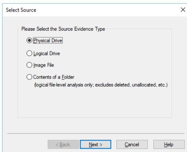
**Figure 5:** Selecting Source Evidence Type in FTK Imager
