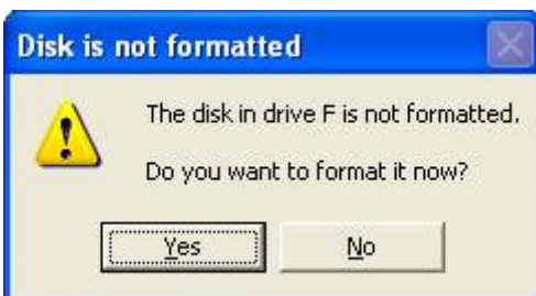
Figure 3 Opening exFAT media in Windows Explorer on an XP system without the exFAT drivers
