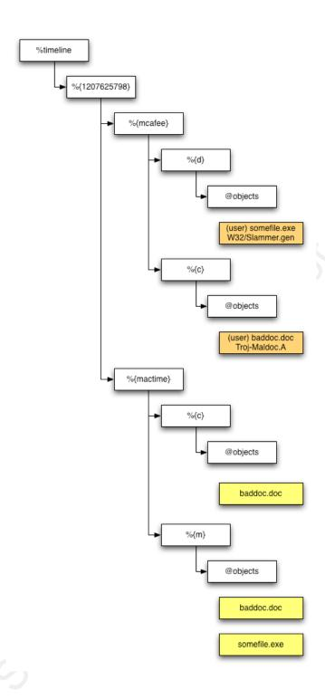
Figure 4: Example hash structure for a file deleted by McAfee
