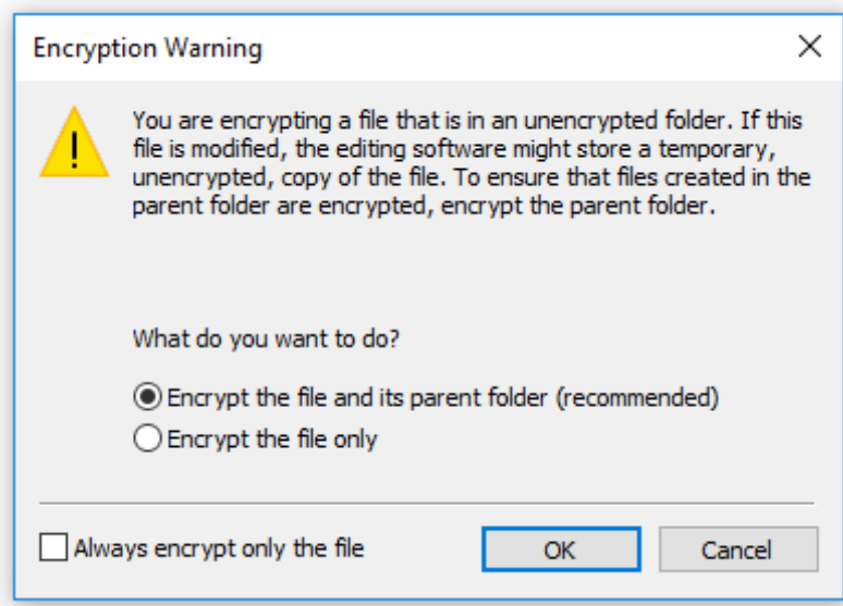
Figure 6-2: EFS warning about application behavior during encryption
