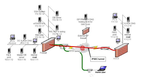
According to the proposal, the GIAC firewall is built on RedHat Linux, using kernel version 2.4.18. The NetFilter (IPTables) kernel module is providing stateful packet filtering.
