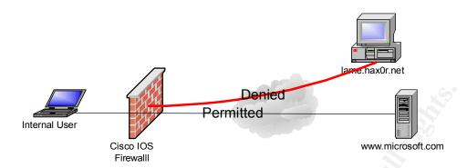
Because no external connections are permitted to protected hosts behind the firewall; connections from www.microsoft.com were permitted to the internal user as those connections were initiated by the internal user. The connection attempt from lame.hax0r.net to the internal user was denied as it was not inititated by the user, the connection attempt was also logged.
