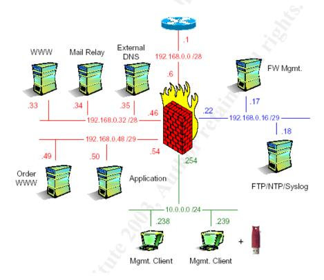
The firewall used in Wolfgang's design is a Checkpoint VPN-1/Firewall-1 Next Generation Firewall version FP3 with Hot Fix (HF) 1 installed. It is running on a Linux RedHat 7.3 server which has been is installed using the checkpoint guideline "Minimum OS Installation Guidelines for Linux VPN-1/Firewall-1
