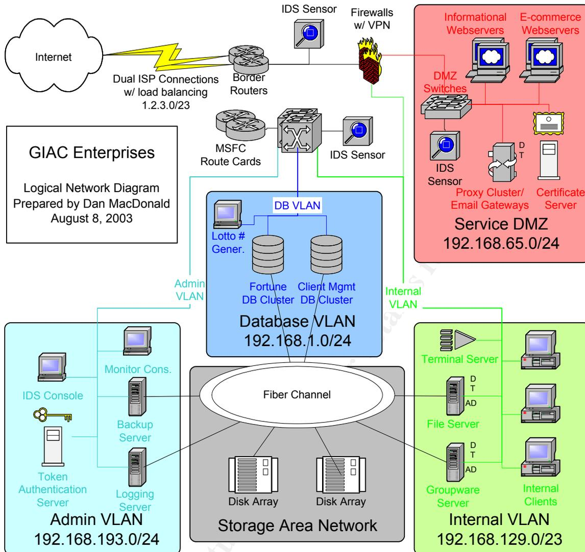
As shown in the above diagram, the network will consist of four LAN segments and one SAN segment inside the firewall: one physically disparate segment, three segments logically defined by VLAN, and one fiber channel SAN.
