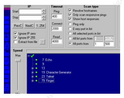
On the following screen, the small services are now deactivated. Only a telnet access is available (for our tests, telnet will appear. The router used is remote to our location and disabling telnet was not an option). Our router will only have console access.
