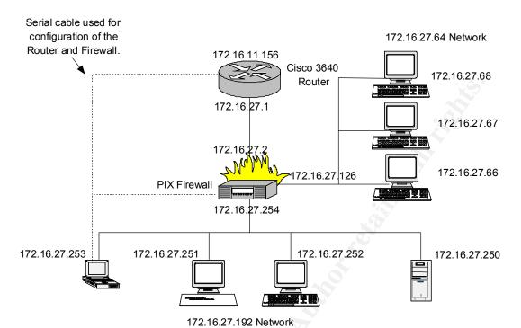
The 172.16.27.156 gives connectivity to the internet via a switch. The interfaces on the router are fastethernet1/0 (address 172.15.11.156) and ethernet2/0 (address 172.16.27.1). The interfaces on the firewall are called outside (address 172.16.27.2), screened (172.16.27.64 network), and inside (172.16.27.192 network). The hostnames of the router and firewall are perimeter and pixfirewall respectively.
