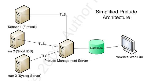
The above diagram is an example of a simple installation of Prelude with a single Management Server and three sensors. A Sensor is any device that reports logs to the Prelude Management Server. Any of the following could be considered a sensor IDS, Firewall, Syslog Server, Workstation, or any other logging device. Prelude can receive logs by directing the device to log to Prelude-LML, using the native compatibility link, or using one of the Programming Frameworks to
