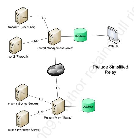
Installing Prewikka on the Management Servers at each site would allow the local Security Personnel to view the current events at their site. Analysts at the central location would be able to view all events from each site reporting in. This setup would be the desired configuration for organizations that are interested in having a dedicated SOC to monitor the events in real-time as well as keeping the local personnel up to date with current events.
