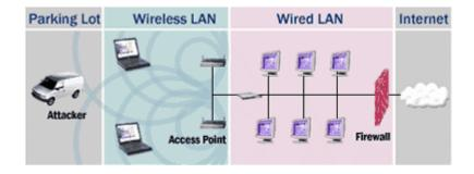
In the above diagram, from <a href="www.airdefense.net">www.airdefense.net</a>, we see the danger that improperly placed access points can have on a network. The access points are connected directly to the internal network and may possibly be granting unauthorized access to an intruder positioned outside in the parking lot.
