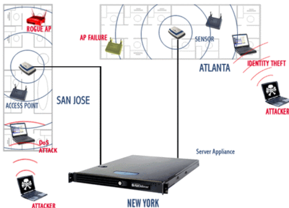
Figure 2. Sample AirDefense IDS diagram [1].
