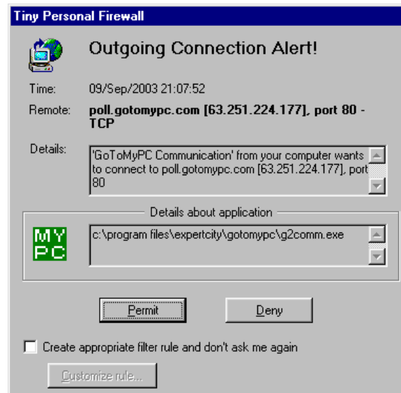
Figure 3 Detection of outgoing connections from GoToMyPC
