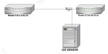
While in this example I used a hub, there is no reason to believe why no switch or tap was used. This is also a possibility, but in such case, it may be true that actually two interfaces were used on the IDS system (to capture both transmitted and received traffic).
