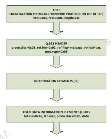
Here is a sample packet capture of an H.225 initial Call Setup:
