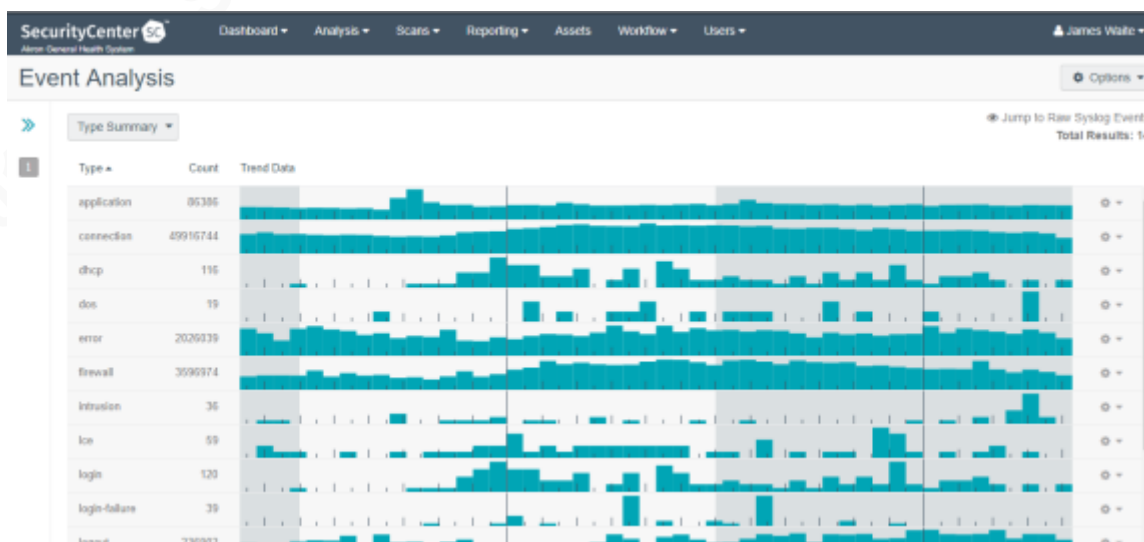
Figure 8 Screen shot of a logging system able to decipher and correlate native and foreign system logs.
