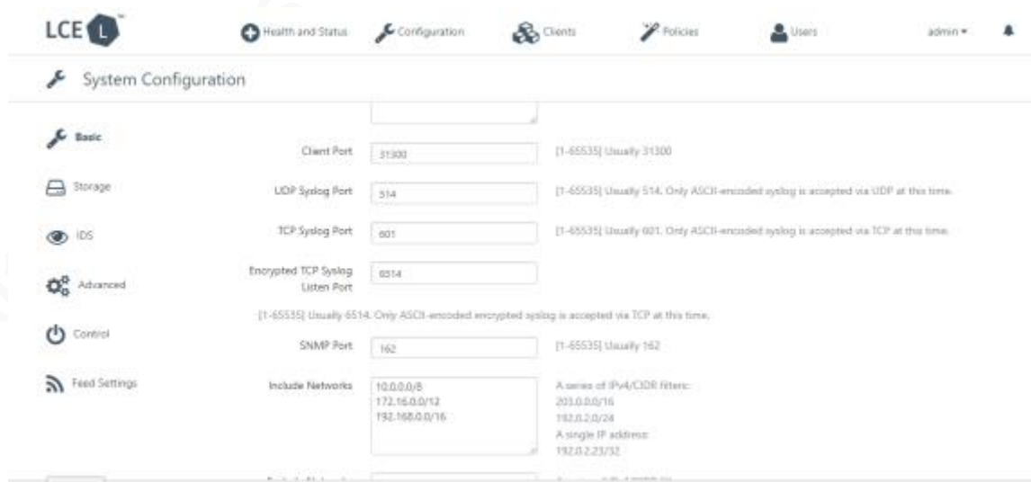
Figure 6 Screen shot of a logging system able to receive and decipher SYSLOG data natively.
