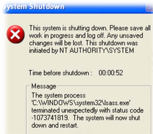
Figure 3-5: A crash in lsass.exe caused by supplying wrong set of addresses to iam.exe
