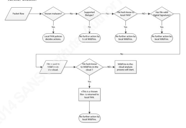
WildFire-in-the-cloud receives unknown files for further analysis. Sandboxing is used to execute the unidentified file in a controlled environment. Its behavior is observed before, during and after the unidentified file is executed. What the file does when executed determines the verdict. A benign file will be reported as such and becomes known as an identified file.
