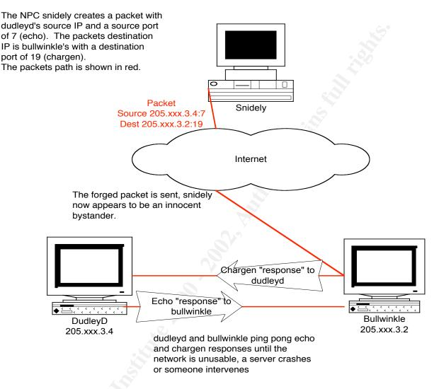
The diagram above shows the original UDP flood vulnerability. The NPC snidely crafts a packet and releases it on the Internet. The unsuspecting victims respond to the packet and ping-pong responses until something breaks or the problem is noticed.
