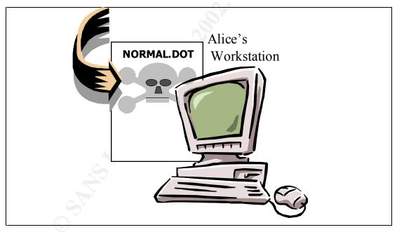
This exploit would also work under Word 2000, although the reasoning is different. In the case of a default Word 97 installation, Word will not warn the user because the macro is attached to a template. In the case of Word 2000, Word will not warn the user because the file is placed in the location that is trusted by default.
