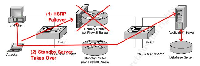
There is no longer any firewall protection for the data center network, and Attacker is free to use traditional tools and techniques to hack into the systems.
