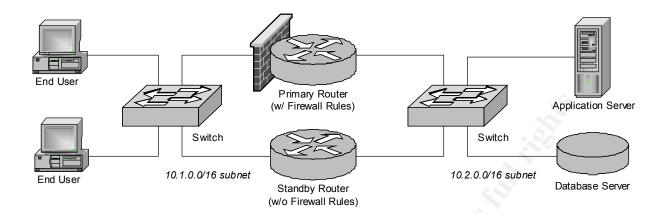
HSRP was tested extensively before installing the standby router, to ensure it works properly. Unfortunately, the network administrator was rushed and therefore forgot to setup firewall rules on the standby router before installing it!
