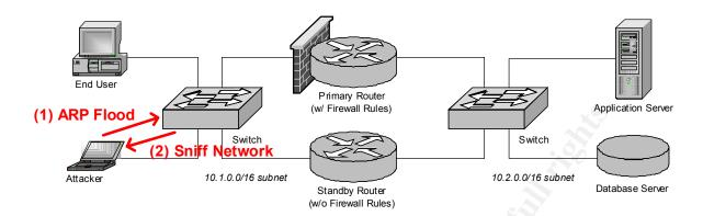
Since all of the valid MAC addresses for devices on the network have been flushed out of the cache, the switch no longer knows how to route the packets and therefore degrades down to behaving like a hub, forwarding copies of all packets it receives into all of its ports.
