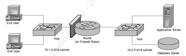
Since the data center network was protected behind a firewall, the IT staff felt it safe to use the "r-commands" (rdist, rcp, rsh, etc.) and NFS, reasoning that the firewall implicitly blocked ports 513 (rlogin), 514 (rexec), and 2049 (NFS).
