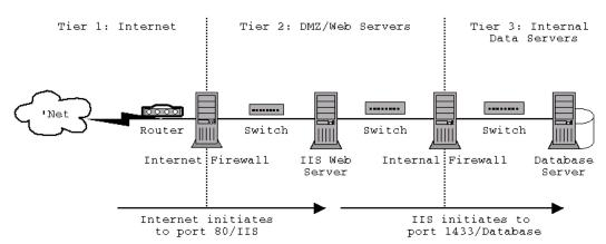
The Internet Firewall only allows connections to be initiated from the internet to port 80; it forwards these packets onto the IIS web server, and allows packets back out through the firewall for established connections. The Internal Firewall similarly only allows connections initiated from the IIS server to port 1433, which it passes to the Database Server. Because of this there is no way for a host on the Internet to initiate a connection to the Database Server.
