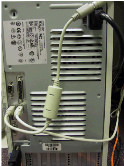
Keyboard cable with KeyGhost installed
