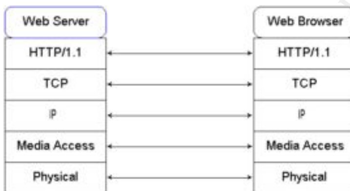
Figure 4: Layer Diagram for HTTP Protocols
