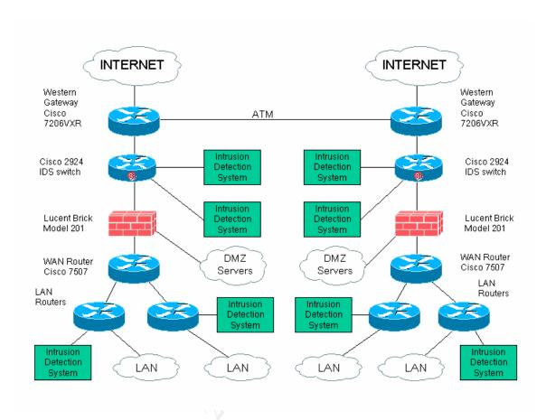
Gateways - Cisco 7206VXR with Enhanced ATM port adapter PA-A3-OC3SMI Cisco IOS version 12.2(7b) with Software Feature Set for IPSEC 56
