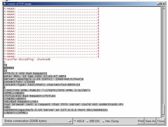
The attacking system will display the following, and an established connection is on the web server from port 32823 of the attacker. Again notice the new "retaddr" after each unsuccessful attempt to get a shell.
