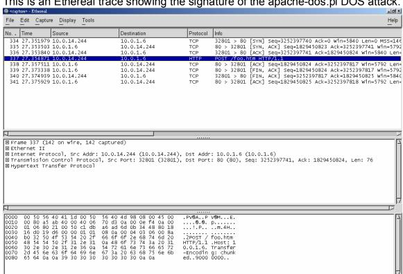
This is an Ethereal trace showing the signature of the apache-dos.pl DOS attack.
