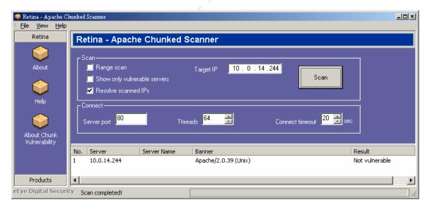
The following is a Ethereal trace of both a vulnerable and non-vulnerable scan from Retina's Apache Chunked Encoding Scanner
