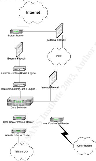
The external and internal Firewalls are Cisco PIX 525s, the cache/proxy engines are Cisco 500 series, and the Core Switches are Cisco 6500 series running IOS version 6.3(3a) with installed MSFC modules running Cisco IOS 12.x. Where possible, the Intrusion Detection probes are integrated into the Catalyst 6500 switches. The firewalls will be configured to allow all traffic in the outbound
