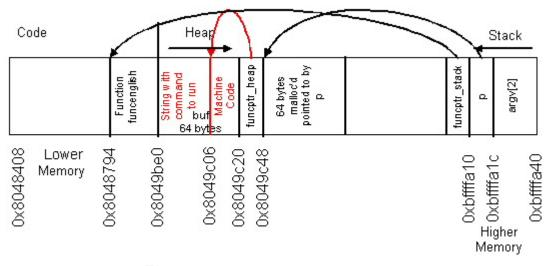
The parts in red are the modifications the program makes to memory which alters the flow of the program. By writing 68 bytes into buf the program overwrites the funcptr\_heap with the location of the code the attacker wishes to run (0x8049c06). Below is the output from running the program and the maillog entry showing the attempted e-mail.
