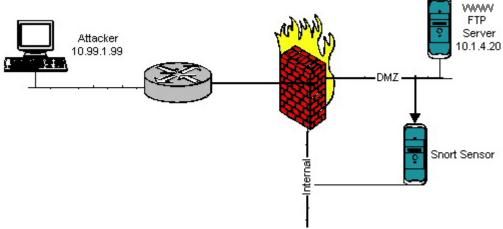
The attacking machine is on a separate box connected to the virtual network through a Cisco 2621 router. The configuration was tested with two different firewalls – the first was Linux Redhat 7.2 using ipchains and the second firewall
