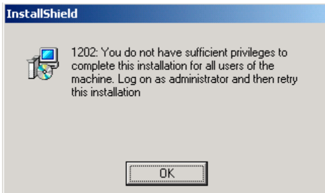
Image #5: Insufficient install privileges
