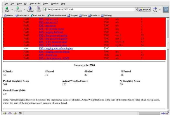
The report also includes a "Fix Script" for making the recommended changes. I print the score report and fix report and use them as a guide to fixing the configuration on the 7500. Many of the changes have to do with tightening security on router access and adding passwords to the terminal lines, and turning off unneeded services. It also shows that I should have this router logging to the external syslog server.
