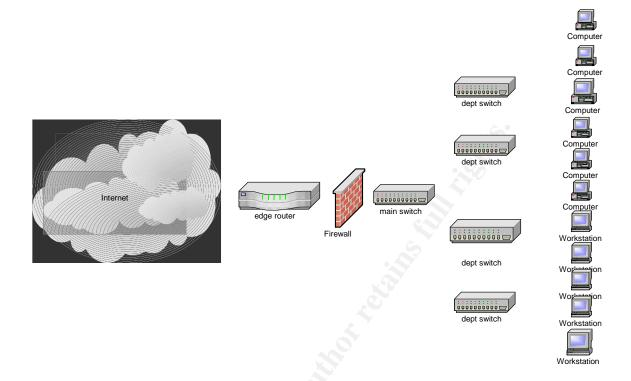
As seen above we have the internet, as shown by the cloud. Then there is the universities edge router, or first entry point if you will. Behind the edge router is a firewall, which in turn leads to the main switch. Hanging off of the main switch are the various departmental switches. Though they are only four listed here there in reality there would be one for each department such as History, Science, and so on.
