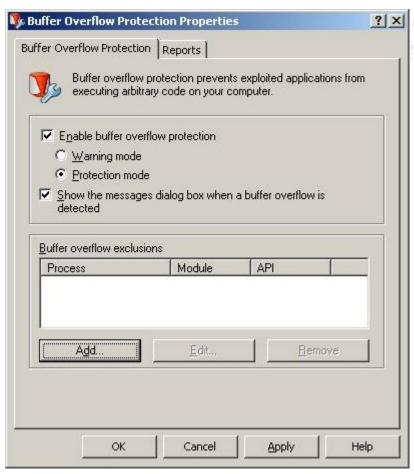
Next, the first virtual machine without VirusScan will be manually infected with Korgo.P so it will attack the second virtual machine with VirusScan. The following screenshot shows the popup message window indicating the buffer overflow was detected and prevented.
