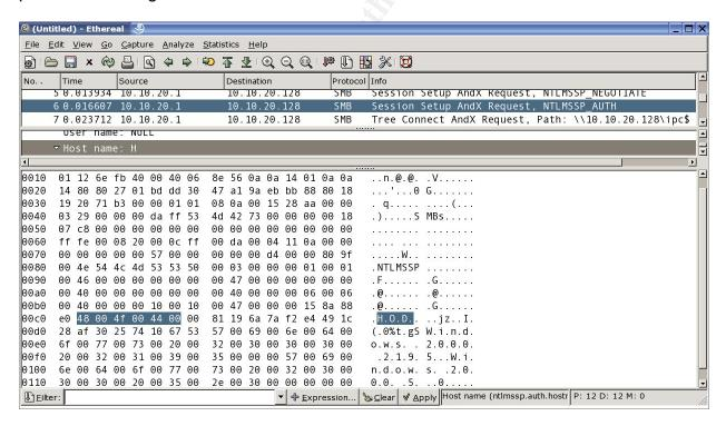
Ethereal Capture showing the compromise by Korgo.P and the highlighted packet containing "HOD."
