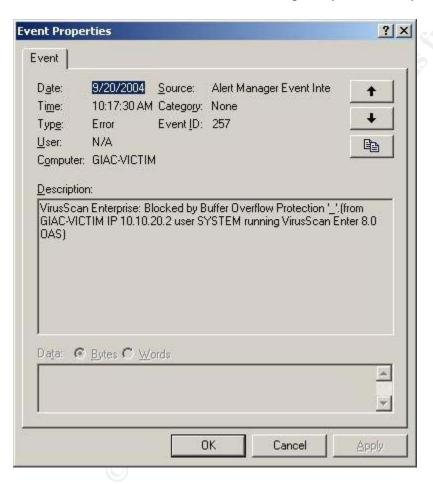
The last test is to verify that VirusScan will also prevent the buffer overflow caused by the HOD exploit code that Korgo.P is based. The following command from run from the host Linux shell.
