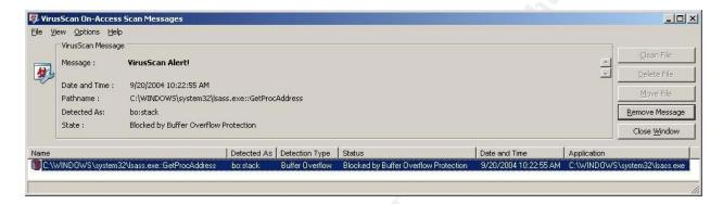
It is interesting to note the difference in API that is listed as the source of the overflow. In Korgo.P, "Isass.exe::GetProcAddress" is listed while HOD shows "Isass.exe::LoadLibraryA." Either way, it is a significant advance in protection to have a piece of antivirus software that can properly detect and prevent a buffer overflow. If only Logan's department had already installed it on all of their computers.
