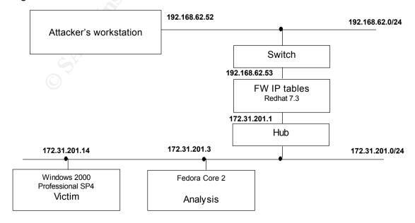
The Analysis server runs a variety of tools (e.g. SNORT, cheops-ng, ettercap, ethereal). A Hub has replaced the Switch in order to make it easier to capture packets on the subnet. The Attacker's workstation has been connected to the 192.168.62.0/24 subnet.
