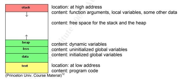
Size of text, data and bss segments doesn't change after loading. Heap and stack have dynamic size so they consume the memory space locates between them.
