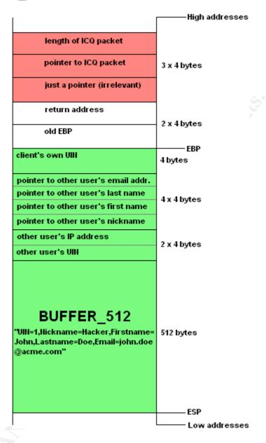
ICQ\_server\_answer\_parser calls ICQ\_command\_processor for each command (embedded subpackets) in the SRV\_MULTI packet. After the last command is processed ICQ\_server\_answer\_parser checks the IP address data from the proper local variable. If it's not null (0.0.0.0) the function fills BUFFER\_512 based on the following C-style code and then finishes its run executing a 'return' instruction:
