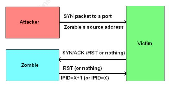
Third step: It's the same as first step. Now we can check the change of IPID. If IPID=X+1, the port is closed or filtered. If IPID>X+2 scanner have to repeat the
