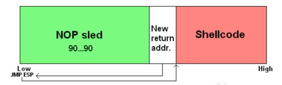
In a typical stack overflow attack, NOP sled could be used with shellcode continuously to provide sure execution if the attacker couldn't calculate a precise return address. In this case NOP sled has only the role of filling the gap. Witty worm used another structure without a NOP sled:
