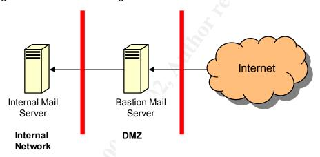
The bastion mail server will reside in the network's DMZ, which is one step from the Internet and considered "untrusted" to the protected internal network. Rules in the firewall and routing software between the DMZ and the internal network will only allow specific protocols to pass from the bastion mail server to the internal network. The protocols that would be required are:
