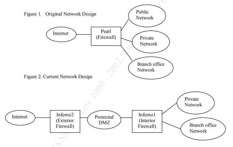
This perimeter defense design is superior because it allowed different firewalls with different responsibilities. The exterior firewall (Inferno2) protects the Internet servers on the DMZ from general access from the Internet as well as defense in-depth for the second interior firewall (Inferno1) which protects the private network with a more stringent ruleset as well as acting as a NAT gateway to the Internet
