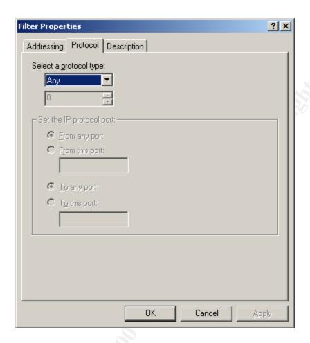
Use the drop-down box to select UDP as the protocol. Then select the To This Port radio button and fill in 1701 as the port. This is shown below.
