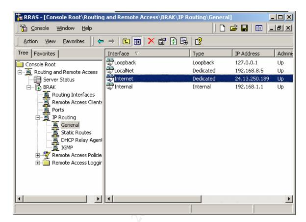
4. Double-click the interface that will accept the VPN connections. (In this example the Internet interface will accept the connections.)
