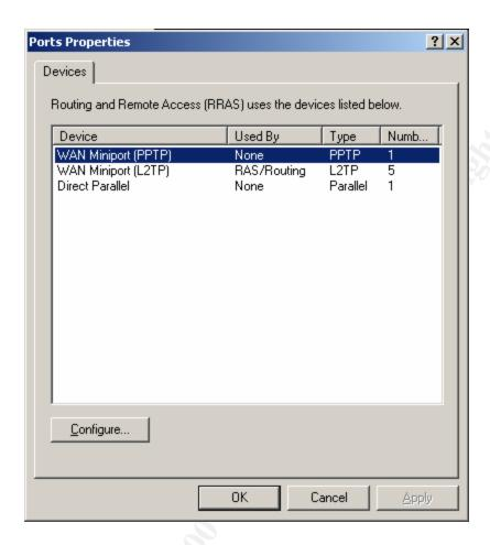
Double-click any of the lines to configure the ports for RRAS access. The L2TP ports should be configured for Remote access connections and Demand-dial routing.
