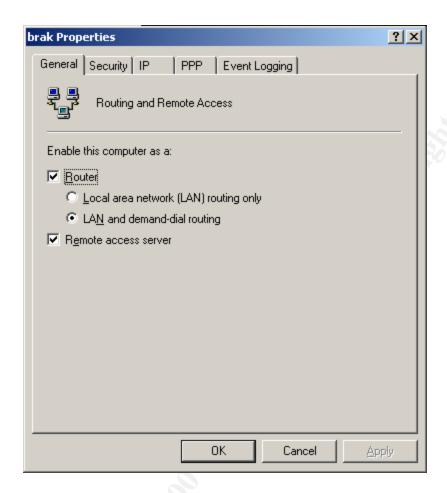
Configure the L2TP server to be a demand-dial router and a remote access server. Then click the Security tab. Clicking the Windows Authentication button will display the following screen:
