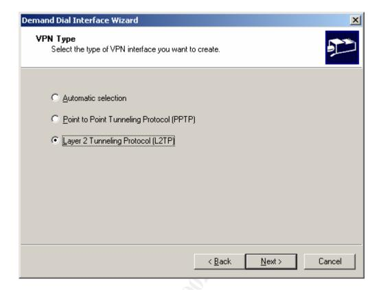
Select Layer 2 Tunneling Protocol (L2TP). The Automatic selection choice is suppose to first attempt an L2TP connection, and if that fails, try a PPTP connection. Based on packet traces of the sessions, selecting Automatic did not initiate any L2TP packets. Instead only data to create a PPTP session was captured.
