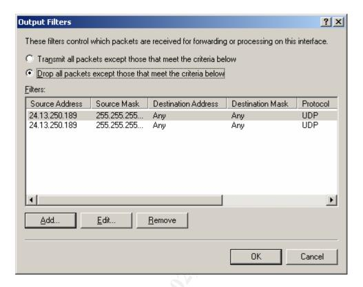
12. Repeat steps 5-11, choosing Input Filters..., instead of Output Filters. Instead of supplies source IP address and port information, provide Destination IP address and port information.
