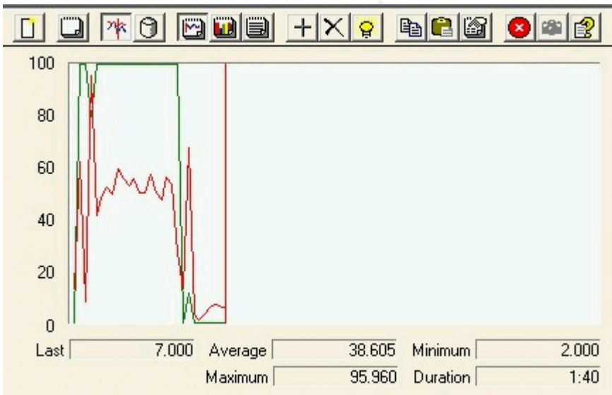
Figure 32 - Laptop file transfer with IPsec and the INTEL NIC - Red line=CPU Green line = Bytes/sec
