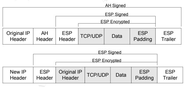
As can be seen, the header and trailer are not encrypted. AH keeps its HMAC in the header and ESP stores its HMAC in the trailer. When the destination device receives the packet it calculates the HMAC and compares it to the HMAC in the trailer. Not encrypting the HMAC allows IPSec to quickly determine if the packet has been modified and, if so, discard the packet.
